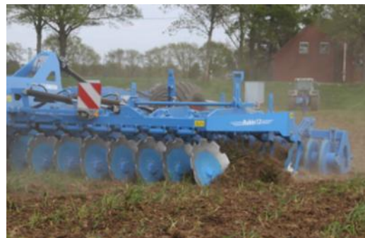
Figur 6.13: Lemken Rubin 12 - aggressive 736 mm tallerkner. Foto: Lemken
